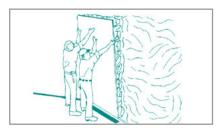
1 • The adhesive is applied on the substrate or on the sheet 2 • The sheet is placed on the substrate
