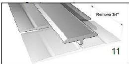
Apply a continuous bead of silicone sealant to both Division Trim Molding channels. Slip under preceding FRP Panel and secure to sub wall. Then, continue with the next FRP Panel. (see illustration 10)
