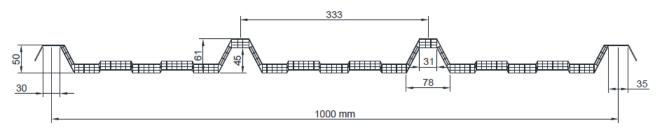
The panel can match various design requiremens due to the possibility to vary the width of the lateral overlapping (upon request). The shape of the overlaps allows side coupling with almost any insulation panels.
