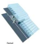
Detail of the panel fixing with hook
